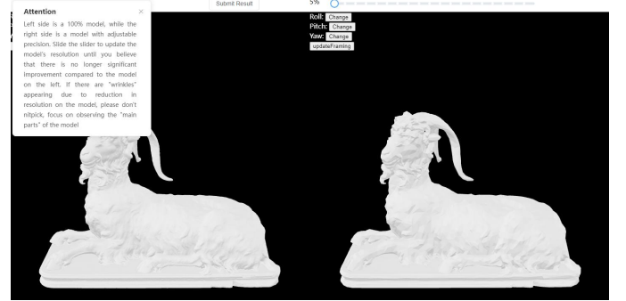
Fig. 4: The screenshot of the comparative experiment system. Both 3D models are in the full body shot. Left side is the original model, and right side is the model after simplification. The two 3D models on the left and right can rotate synchronously. When the participant rotates one of the models, the other would also rotate at the same angle.
